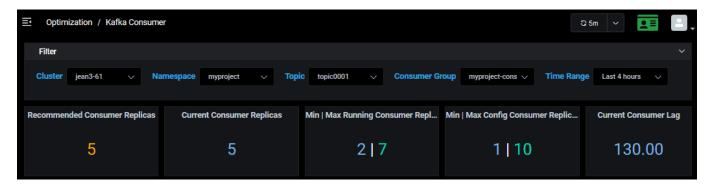
The number of recommended and current consumer replicas is displayed along with the minimum and maximum number of running and configured replicas and the current consumer lag.
