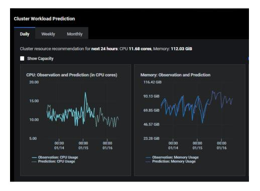
Check *Show Capacity* to see the maximum CPU and memory usage limits for the cluster. Orange represents 80-90% and red represents 90-100%. This is a useful way to see if the utilization of resources is approaching the overall cluster capacity.
