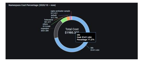
The *Namespace Cost Percentage (Last Hour)* chart displays the actual cost for each namespace and when system was idle during the past hour. The *others* tag represents the unmonitored namespaces in a cluster. Move your cursor over each bar to show the cost of a namespace or when system is idle.
