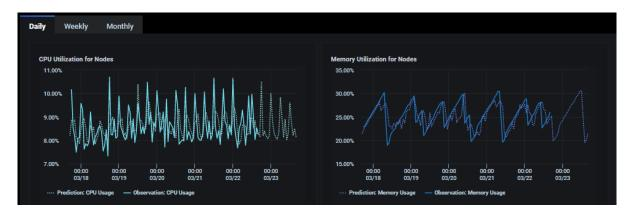
The solid lines represent the observed actual usage while the dotted lines show the historical and future predicted usage. The predicted usage is used in the analysis for cluster configuration recommendations.
