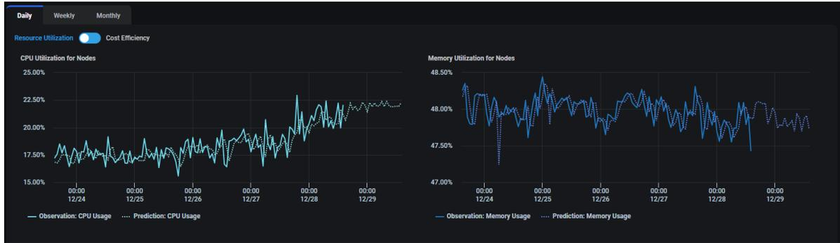
The solid lines represent the observed actual usage while the dotted lines show the historical and future predicted usage. The predicted usage is used in the analysis for cluster configuration recommendations.
