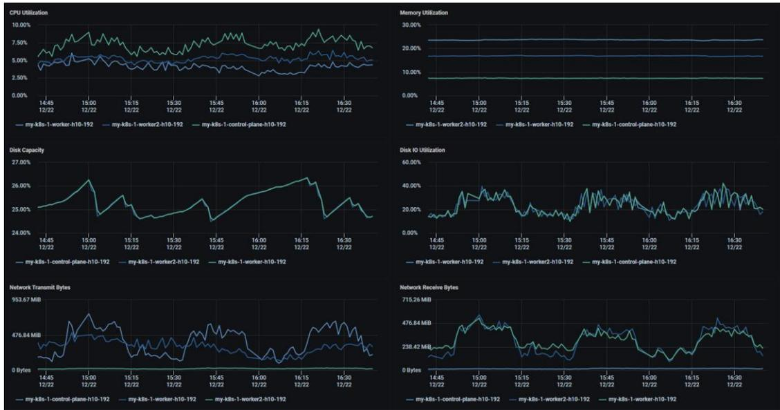
CPU utilization, memory utilization, and network input and output charts are displayed for each VM.
